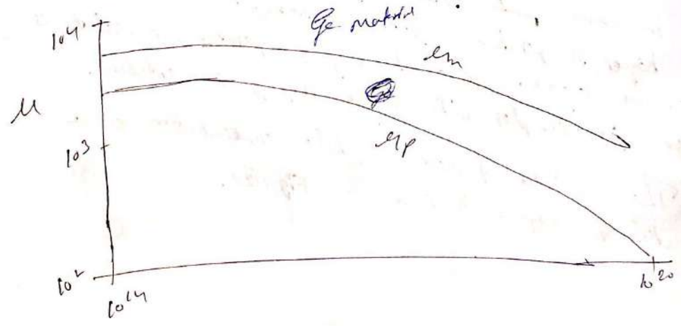
Fig. (12) n & h mobilities in Si at room temperature as a function of impurity concentration.
